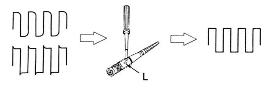
Adjust trimmer L until seeing flat-top square wave on the display.
